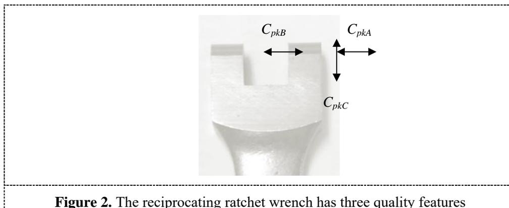
**Figure 2.** The reciprocating ratchet wrench has three quality features
