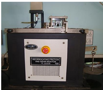
Figure 1. Reciprocating test rig
