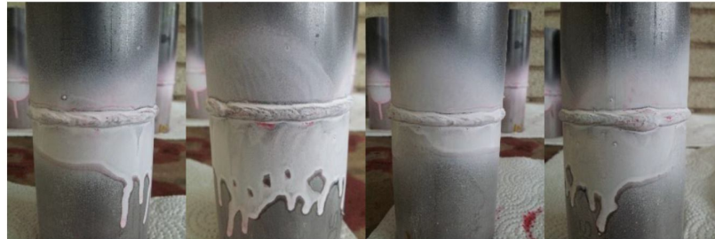
Figure 2. Sample no.1 of TOW with 160 A, 19.25 V and 3 RPM as parameter shows red dots at the start-end.
