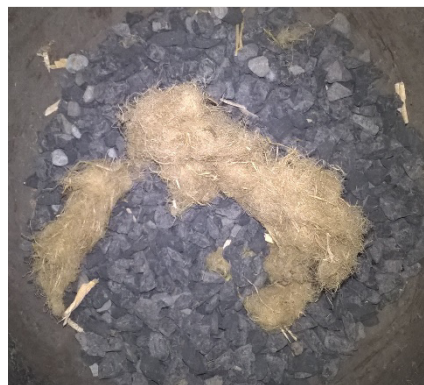
Figure 3. Tufts of raw hemp fibers mixed with gravel.
