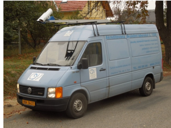
Figure 2. Measuring vehicle with both cameras on roof frame.
