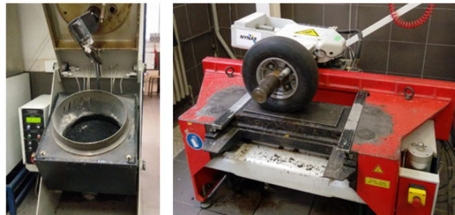
Figure 4. Manufacturing and compaction of the asphalt.
