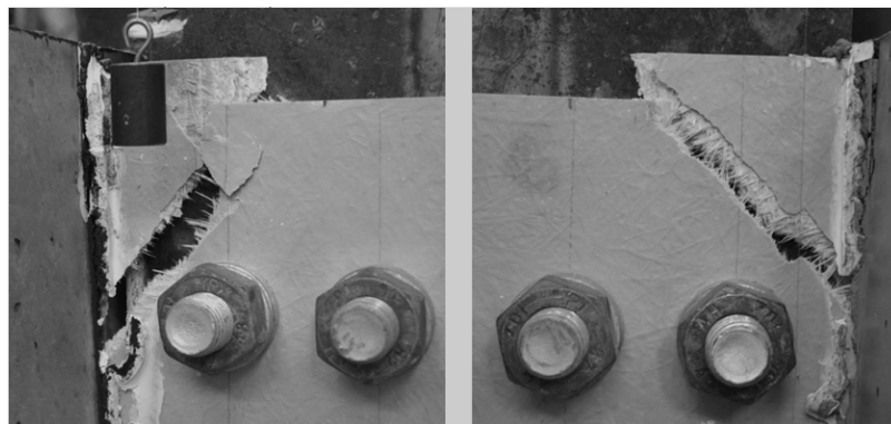
Figure 5. Shear cracks of the push out test specimen.
