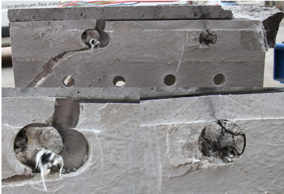
Figure 6. View of the failure of the composite connectors.
