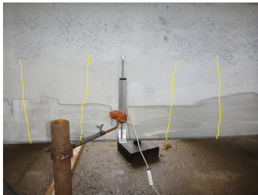
Figure 6. First cracks in the test ( 4 \times 0.1 mm, F = 125 kN).
