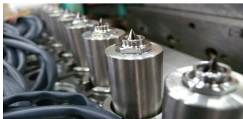
Figure 15. Hot runner gate
