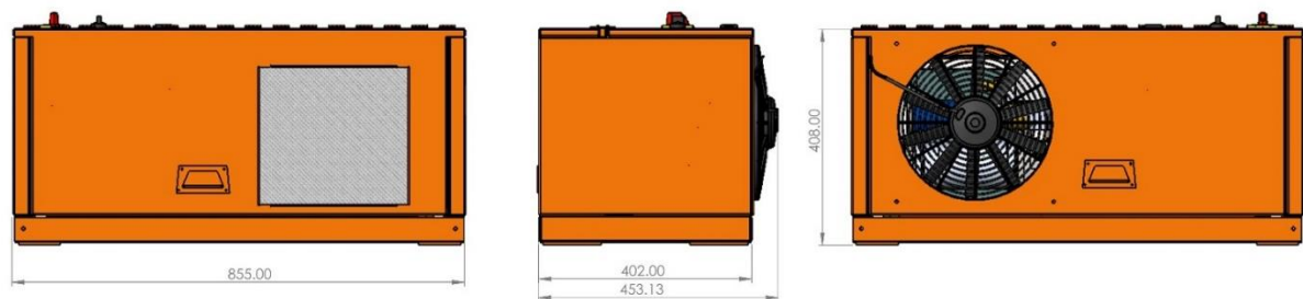
Figure 5. Dimensions of the conical screw compressor VERT.80
