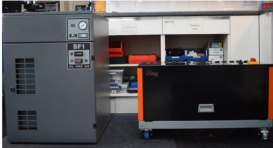
Figure 4. Scroll compressor Atlas Copco SF 1 (left) and conical screw compressor VERT.80 (right)
