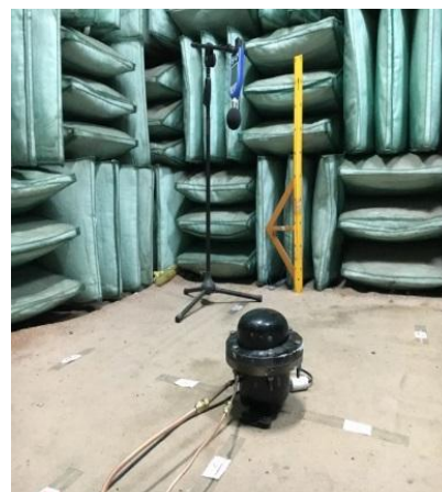
Figure 8. A semi-anechoic room of noise test.
