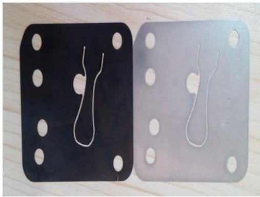
Figure 1. Comparison of conventional and improved suction valves.
