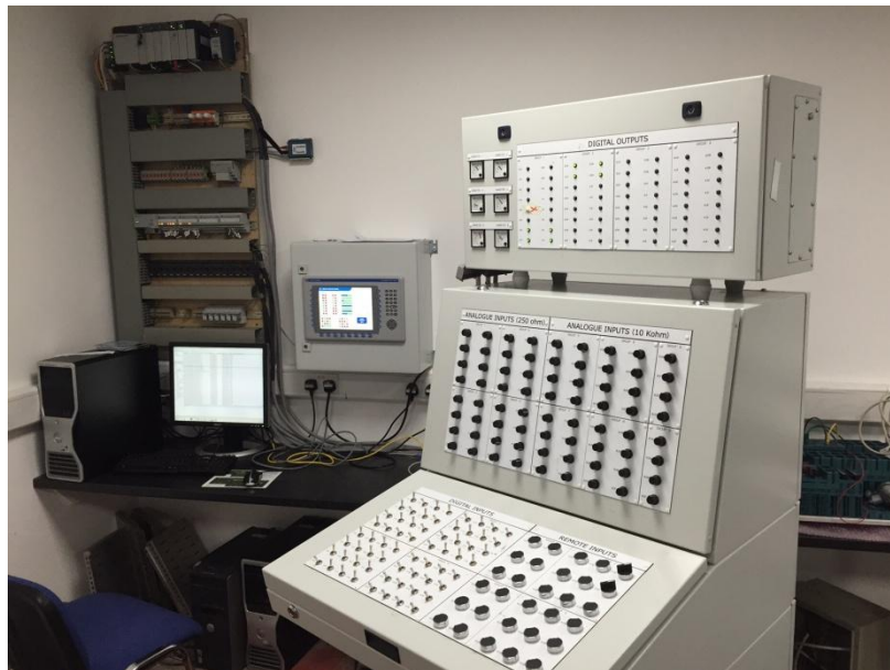
Figure 3, the single node proof of concept test assembly.
