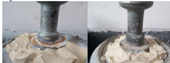
Fig.6: Samples of Corroded Insulators 2# (left) and 6# (right)
