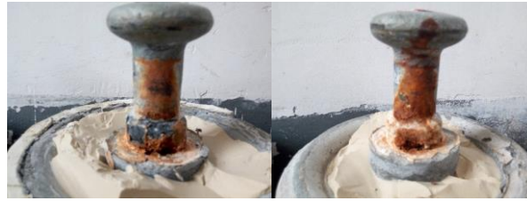
Fig.7: Samples of Corroded Insulators of 3# (left) and 4# (right)
