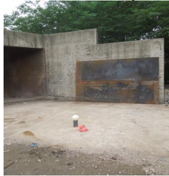
Figure10 The test arrangement of cutting MEFP
