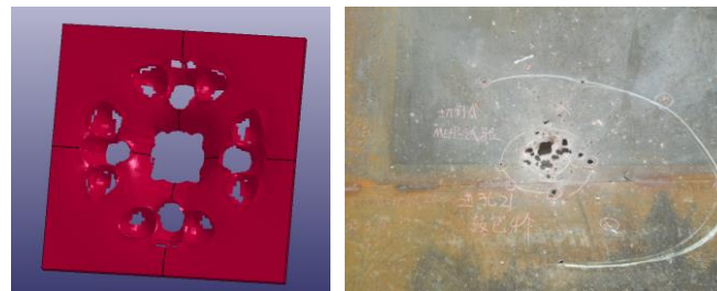
Figure 11 The contrast between the simulation and test penetration
