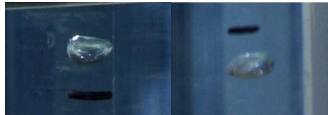
Figure 2. The morphological change during bubble rising behavior
