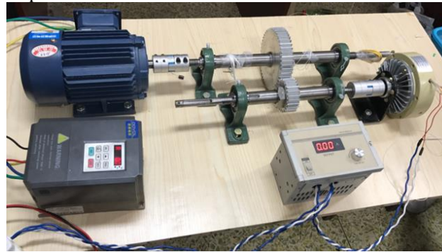
Figure 3 the experimental platform of gear running state detection system
