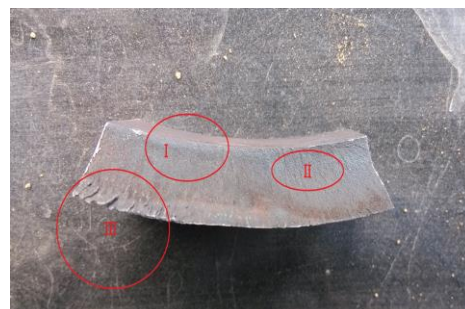
Figure 2 Macroscopic morphology of quenching crack.
