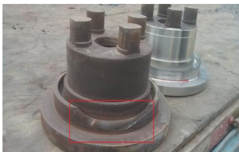
Figure 1. Position and morphology of quenching crack of planetary carrier.
