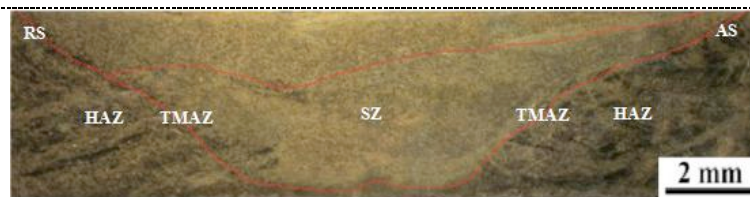
Figure 1. Electronic cross-sectional macro-image of FSPed sample with a rotating speed of 1500 rpm.
