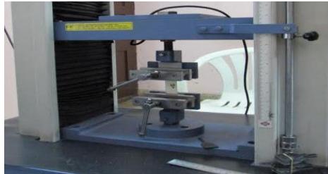
Figure 3. Universal Testing Machine with 20kN capacity
