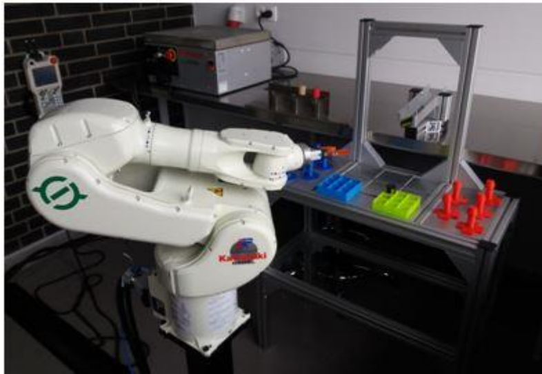
Figure 1. The laboratory of Multimotion Control. The research lab station with Kawasaki RS005L robot.
