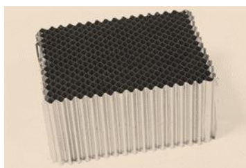
Figure 1. Welded honeycomb structure.
