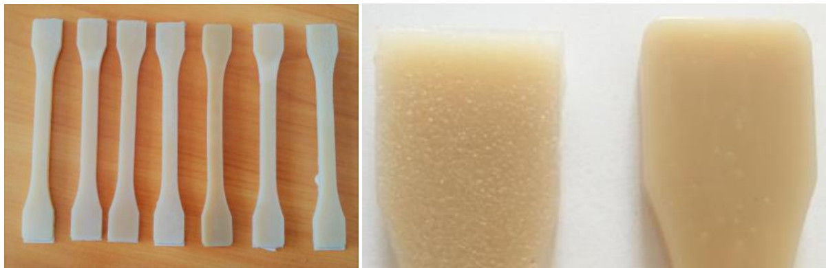
Figure 6. Molded testing samples and differences between two moulding series.
