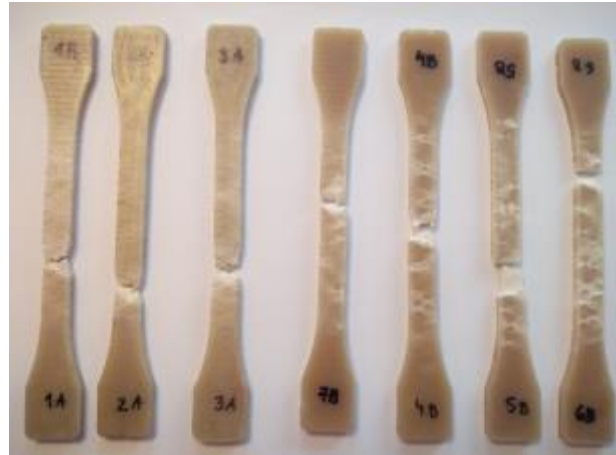
Figure 7. Testing samples after tensile strength tests.
