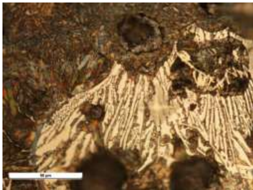
Figure 11. Hard spot in padding weld. Measured point 707 HV 0.5.
