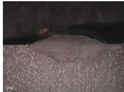
Figure 8. View of microstructure of EB 150 overlay weld.
