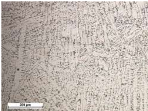
Figure 7. View of dendrites in padding weld ES 18-8-6B.
