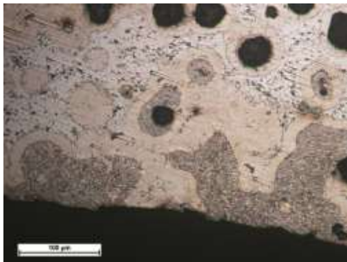
Figure 3. Microstructure of cutting HAZ.
