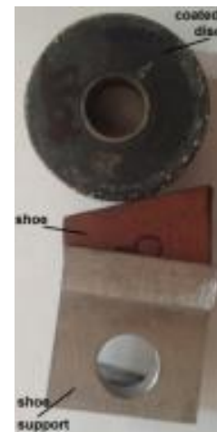
Figure 2. Configuration of roller-shoe contact.
