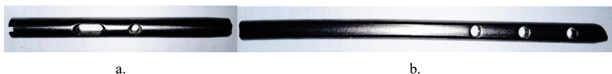
Figure 1. Prosthesis components after removing the flaw: a - superior part b - inferior part.
