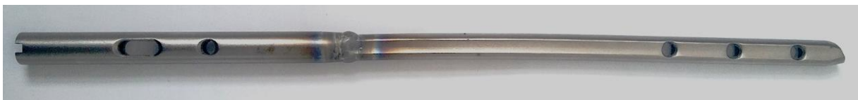
Figure 3. The prosthesis obtained by welding reconditioning.
