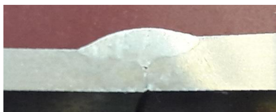
Figure 5. Welding seam macrography.
