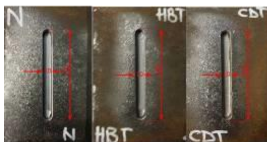
Figure 4. The canals of the N, HBT and CDT samples (canal depth: 10 mm).
