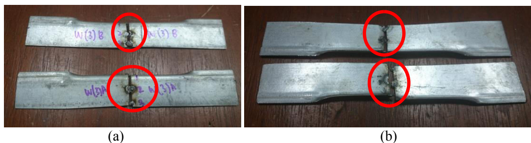
Figure 5. The failure on spot weld for SW3SC specimen (a) front view and (b) back view
