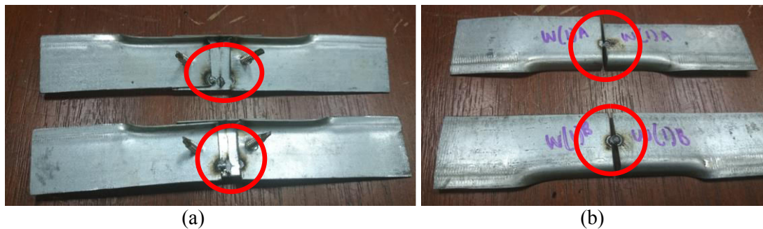
Figure 4. Example of the failure on spot weld for (a) LDWSC and (b) SW1SC specimen
