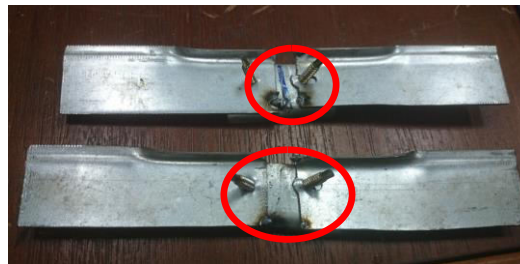
Figure 6. The failure of the self-drilling screw of LUWSC specimen
