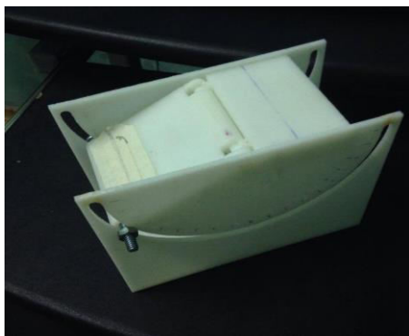
Fig. 6. Customized bending jig.
