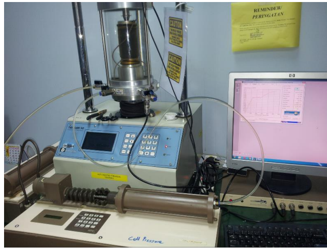
Figure 2. Reconstituted Peat Sample on Triaxial Test Machine
