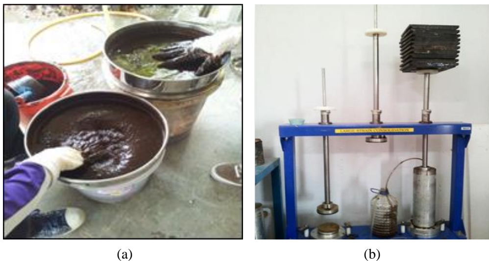
Figure 1. (a) Reconstituted Wet Sieving (B) Reconstituted Pre- Consolidation Pressure
