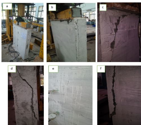
Figure 8 Typical view of cracking pattern of panel from crack initiation to ultimate failure
