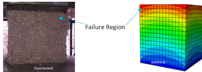
Figure 7 Comparison of failure behaviour of lightweight concrete cubes
