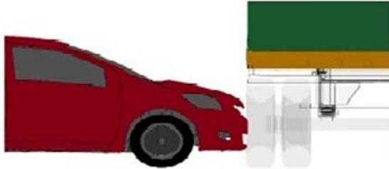
Fig(1.1) Inequality between passenger vehicle bumper and trailer
