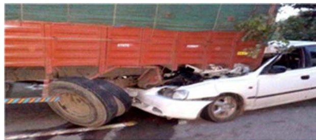
Figure 1.2: The Car Impact with Rear End of Truck
