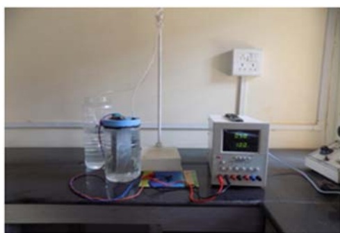
Fig.3. experimental set-up of electrolyzer connected with multiple power supply.
