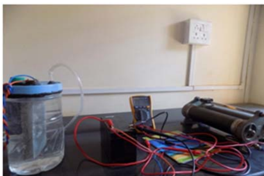
Fig.4. Electrolyzer connected to 10V battery and Rheostat in parallel. The digital multimeter connected in series to
