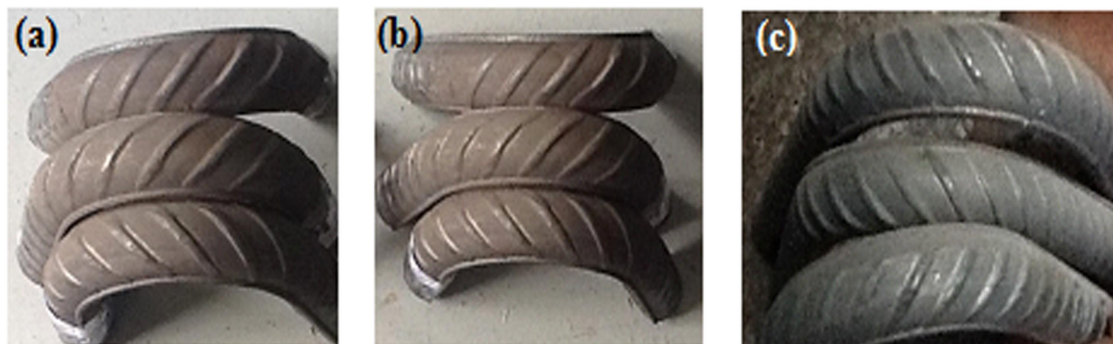
Figure.3 (a) to (c) shows crack free surfaces and without open defects after the bend test.
