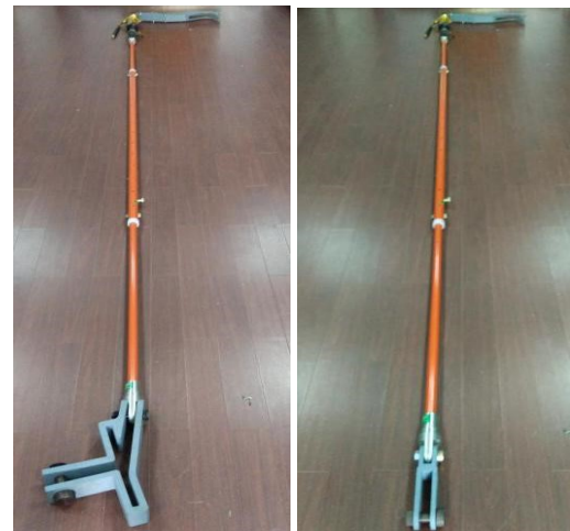
Figure 2. The tools of replacing the L-type insulator string
