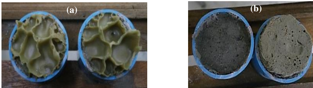
Figure 1. Failure Behavior of Sample (a) Cohesive failure (b) Adhesive Failure (diameter 40 mm)
