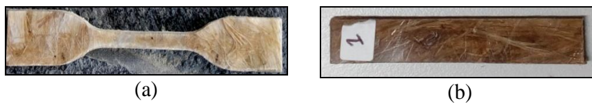
Figure 1. Test specimens: (a) tensile test, (b) flexural test
