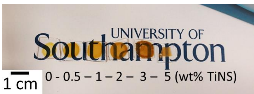
Figure 5. A photograph showing the effect of titanate nanosheets on the optical properties of polyamic acid salt (titanate content from left to right: 0, 0.5, 1, 2, 3, 5 wt%)
