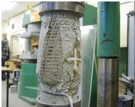
a) overlapping zone z=70 mm, where z/u=0.2 ( u – perimeter of the sample, 113 mm)
