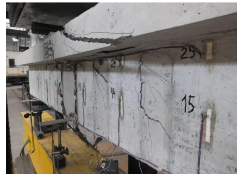
Figure 6. Failure of beam – crack along the bar and PBO debonding
