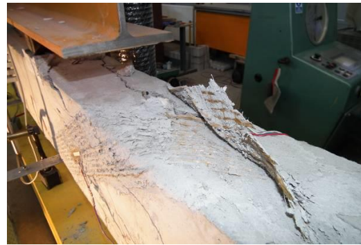
Figure 3. Failure of beam B3 – pulling the endings of PBO stirrups out of the lap
