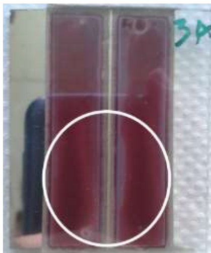
Figure 5. Photograph showing electrolyte leaking observed in the sub-module sealed with Amosil with 1:1 ratio.
