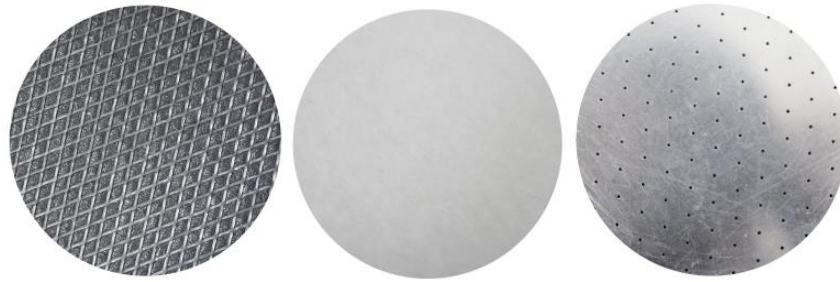
(a) aluminum fibrous acoustic board (b) polyester (c) micro-porous board
