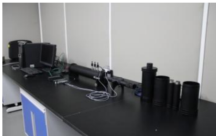
Figure 2. B&K impedance testing system.
