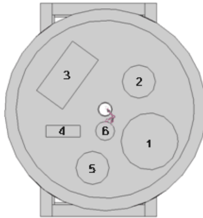
1 the reaction kettle 2 the electromotor 3 feeding equipment and receiving device 4 console 5 transducer 6 CO 2 battery
