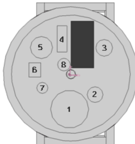
1 the reaction kettle 2 the incoming container 3 the transducer 4 the receiving device 5 the electromotor 6 the feeding equipment 7 the receiving bottle
