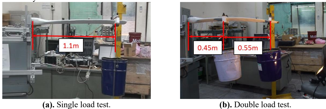
Figure 5. Load-control test of wind blade.
