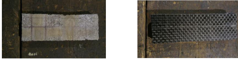
Figure 2. AlSi10 foam (left) and CFRP coated AlSi10 foam (right) materials specimens.
