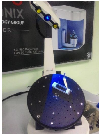
Figure 5. Scanning process by Solutionix Rexscan CS2+ laser scanner
