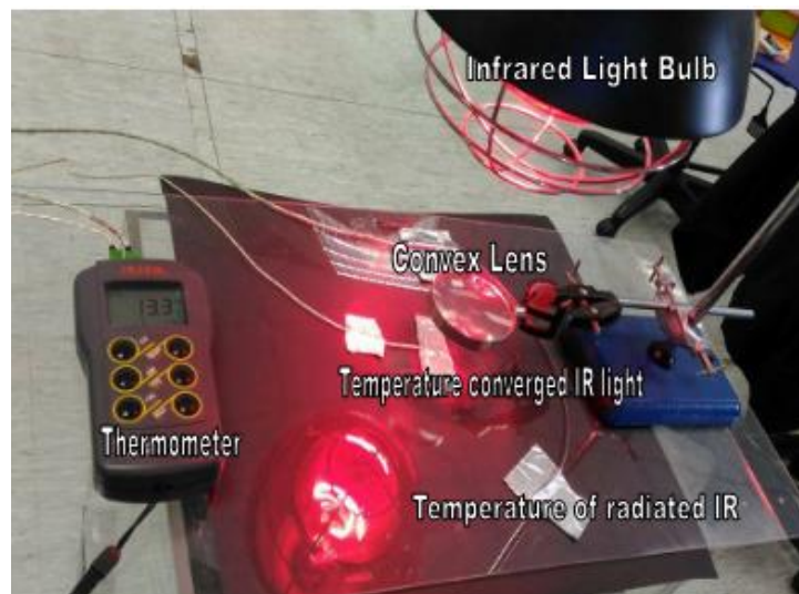
Figure 4. Measuring temperature of radiated IR light and converged IR light
