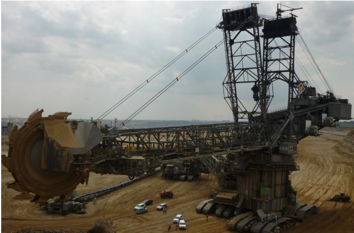
Figure 1. A bucket wheel excavator in the marching position.
