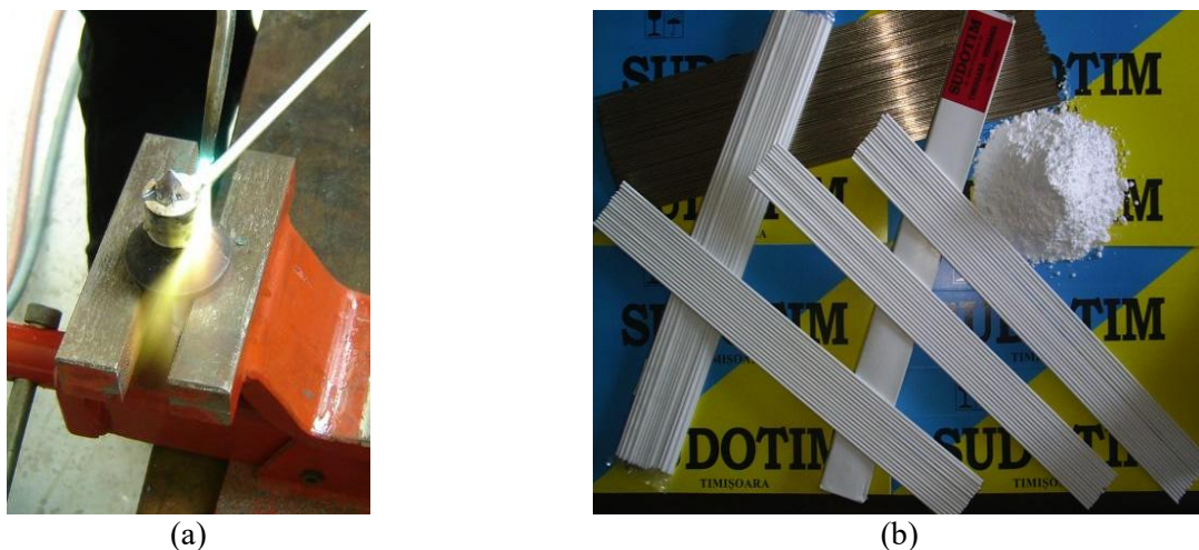
Figure 2. Manual oxy-flame brazing process (a) and filler materials (coated rods) (b).
