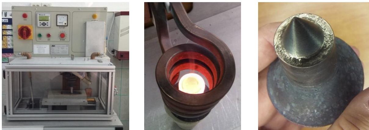
Figure 6. Installation for brazing in protective atmosphere and the brazed assembly.
