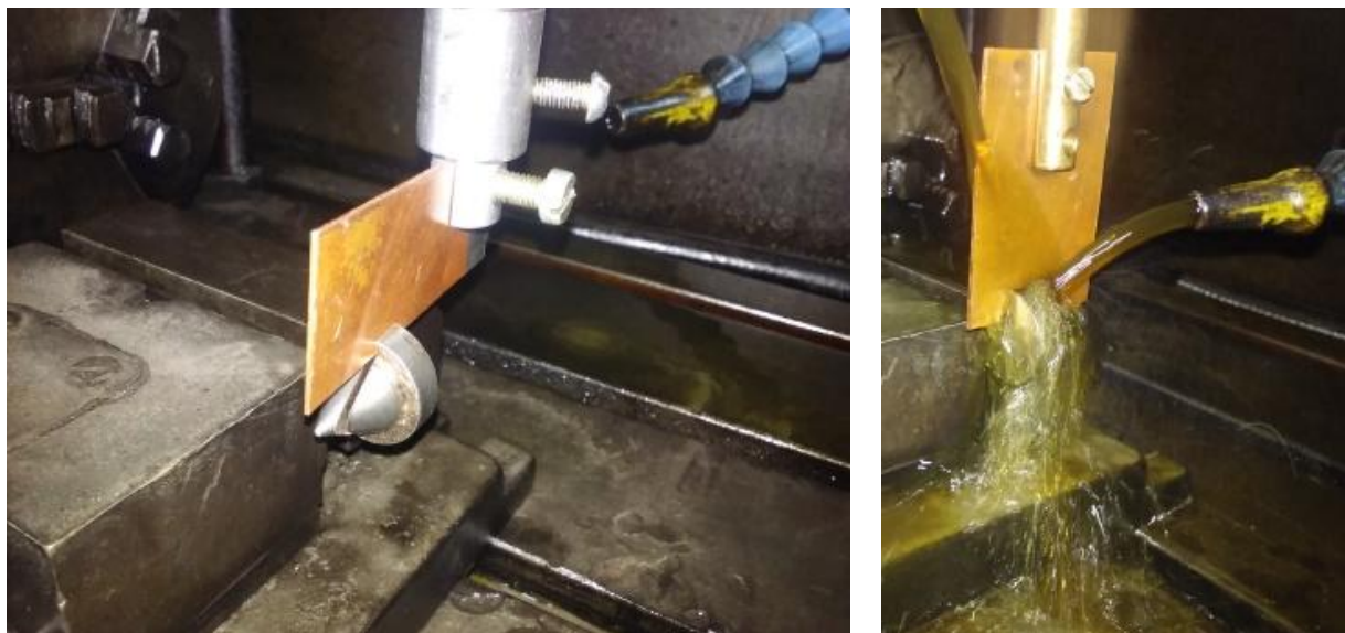
Figure 7. Spark erosion cutting of the brazed assembly.
