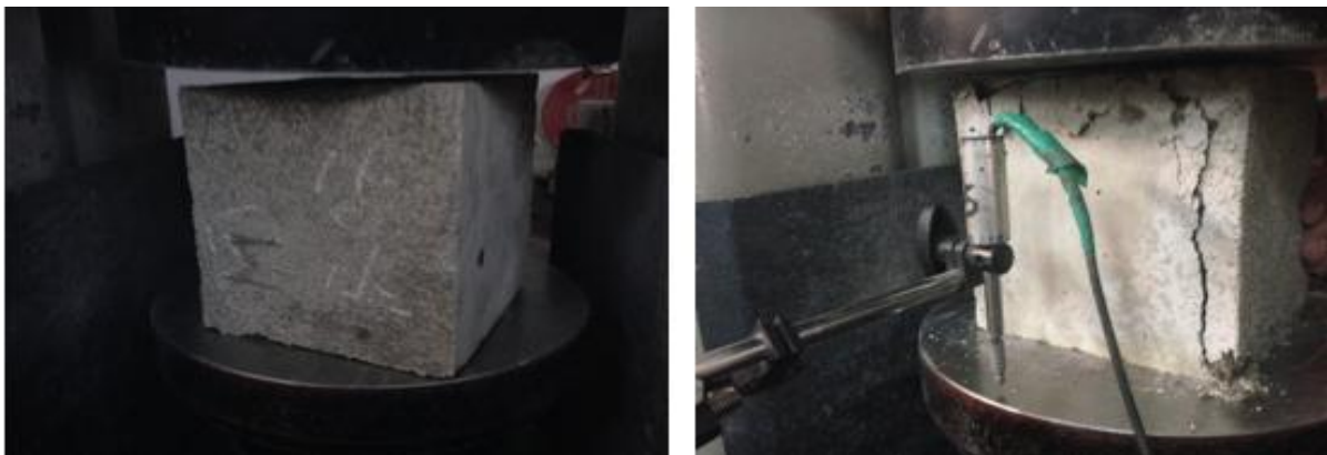
Figure 2. Concrete Strength of the tested specimens.
