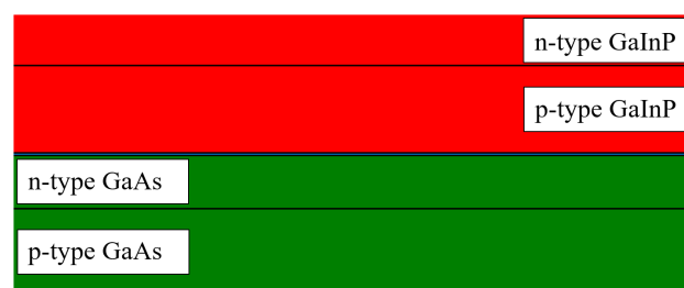
Figure 1. \text{Ga}_{1-x}\text{In}_x\text{P}/\text{GaAs} Solar Cell layer.
