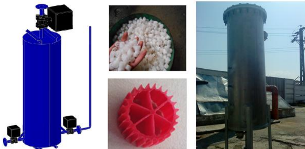
Figure 1. The pressurized capsule for a DAF unit and an example of a plastic element.
